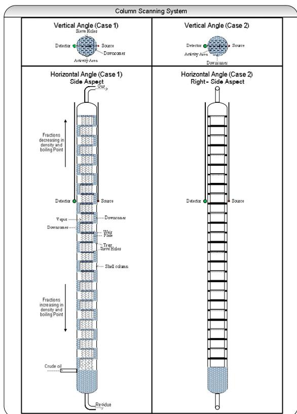
Figure 2 Sample of Column Scanning System
