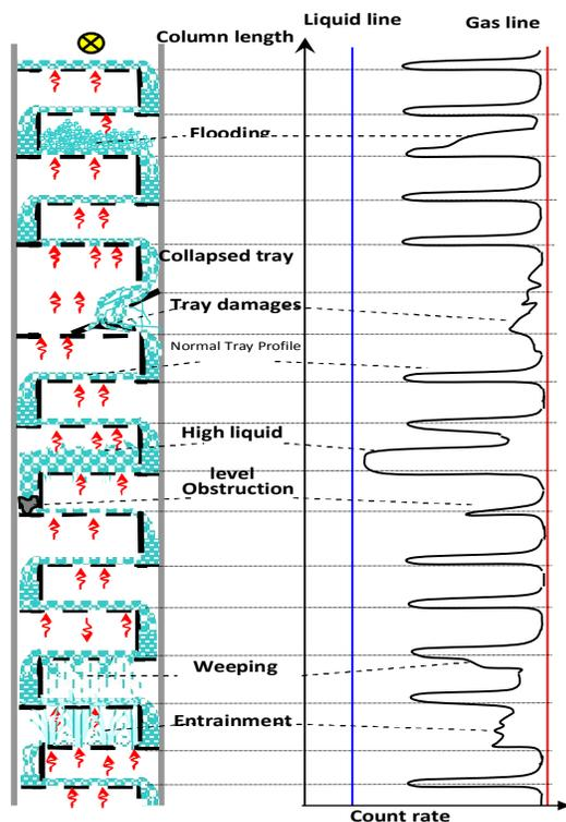
Figure 1: Sample diagnosis patterns obtained by gamma column scanner
