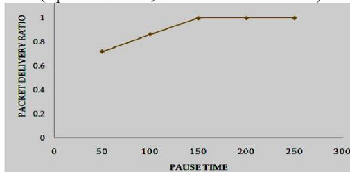
Figure 4. Packet Delivery Ratio Vs Pause Time (Speed=20m/s)
