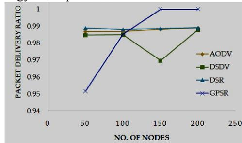
Figure 8. Comparison of Packet Delivery Ratio of GPSR with traditional protocols
