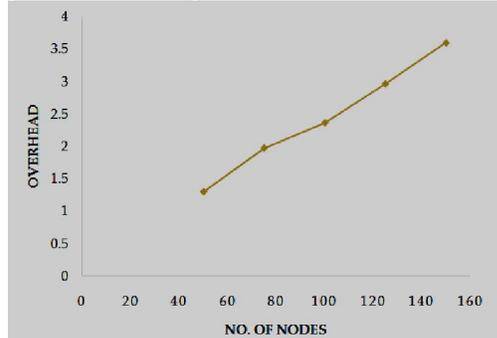
Figure 6. Traffic Overhead Vs Number of nodes
