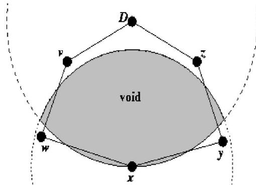
Figure 1: node  $x$ 's void with respect to destination [1]
