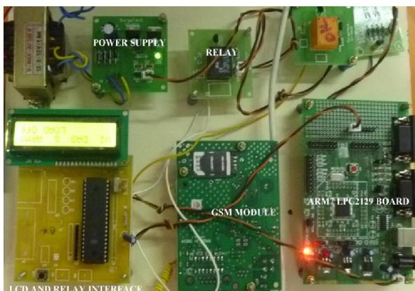
Figure 11. Complete hardware module with GSM modem and Interface circuit module
