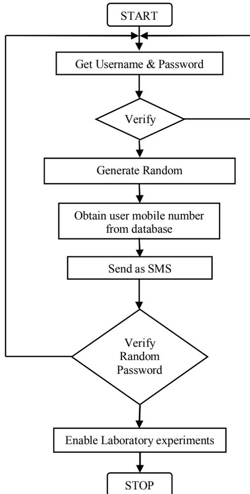
Figure 1. Flowchart Representation of Authentication through Random Number
