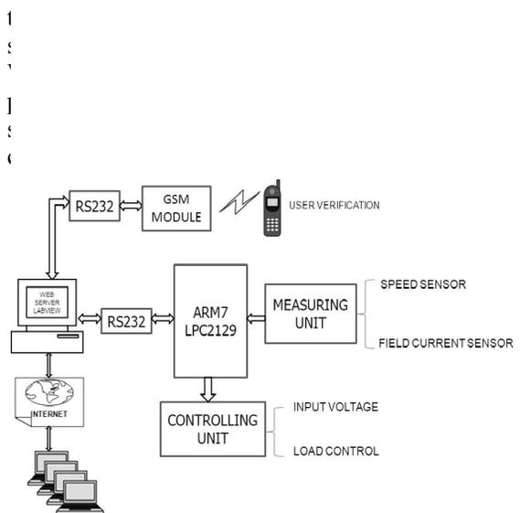
Figure 5. Hardware Implementation block diagram.
