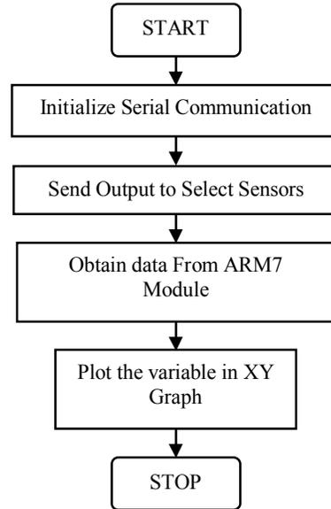
Figure 3. Flow chart representation of data acquisition (ARM7 Module)
