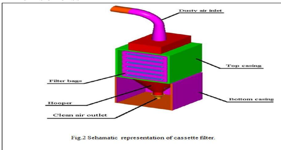
Fig.2 Schematic representation of cassette filter.
