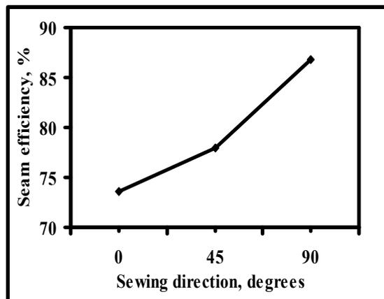
Figure 12: Effect of sewing direction the seam efficiency.
