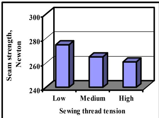
**Figure 3:** Effect of sewing thread tension the seam tensile strength.
