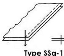
**Figure A:** seam of type SSa-1 used in this study
