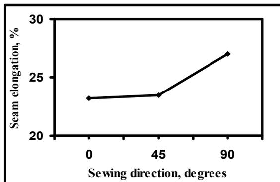
**Figure 8:** Effect of sewing direction on the seam elongation.
