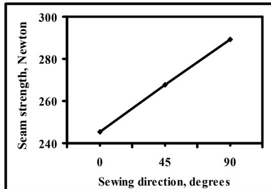
**Figure 4:** Effect of sewing direction on the seam tensile strength.
