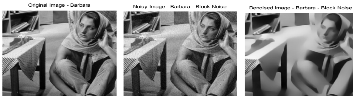
Figure 5: Original image ,noisy image and denoised image by using Lena and barbara (image) for block noise.
