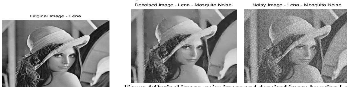
Figure 4: Original image ,noisy image and denoised image by using Lena and barbara (image) for mosquito noise.
