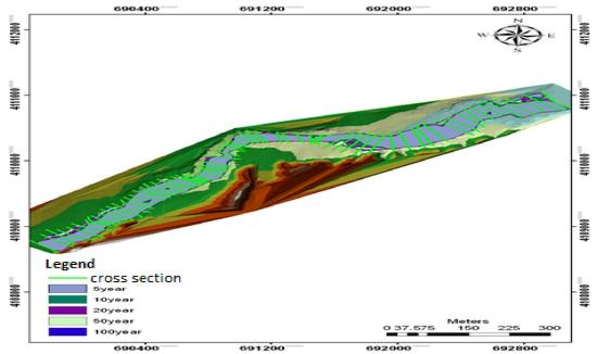
Figure 5: Flood zoning of a part of Ay-Doghmush River using HEC-RAS model and ARC GIS software
