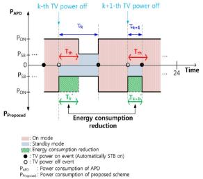
Figure 4. Compare the power consumptions of APD and the proposed scheme.
