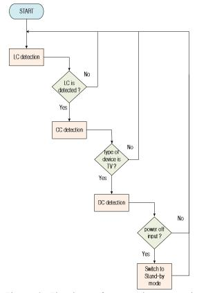
Figure 3 Flowchart of proposed power-saving scheme in STB.
