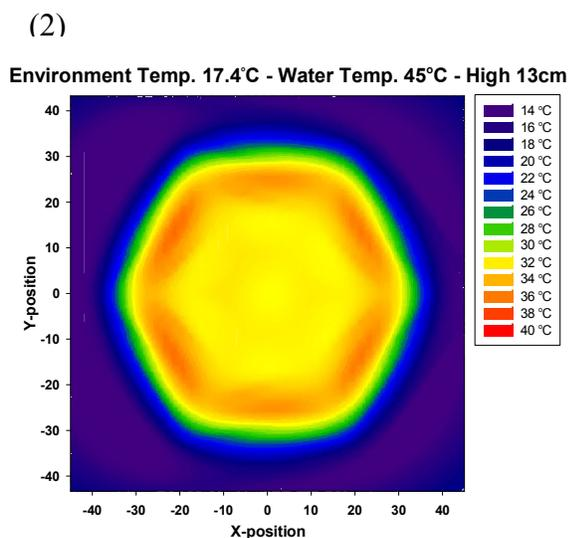
Figure 7. Temperature distribution under the poultry heater, (1) computer simulated, (2) experimental measured
