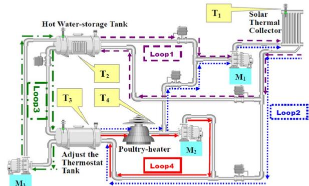
Figure 2. the loops of solar keep warm system
