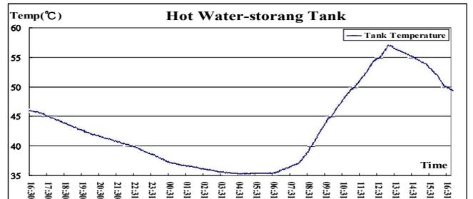
Figure 4. Temperature distribution of storage tank
