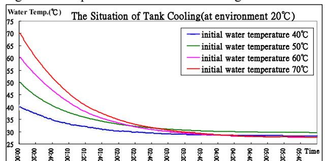
Figure 5. The cooling rate of water without any heat source
