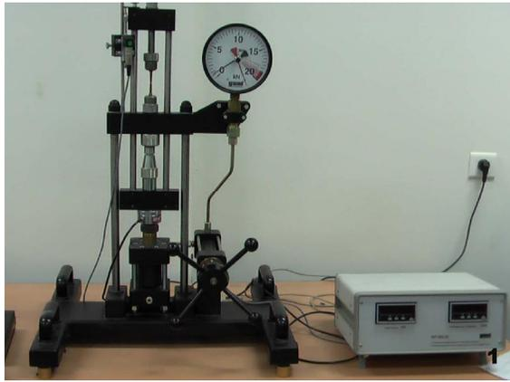
Fig. 1. Photograph of tensile strength machine (Wp 300.20- PC measurement data recording system for universal machine).
