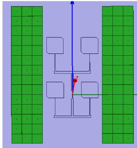
Figure 7. 2x2 Circular polarized antenna with three EBG rows
