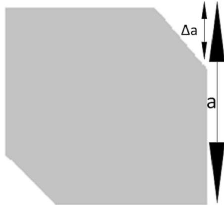
Figure 1. corner truncated patch for circular polarization
