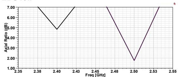
Figure 5. Axial ratio for CP array antenna with (dash line)and without EBG (solid line)
