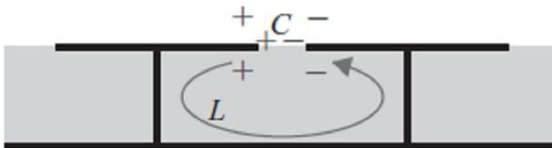
Figure 2. Lumped LC model for EBG
