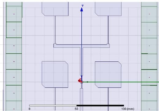
Figure 4. 2x2 Circular polarized antenna with one EBG row
