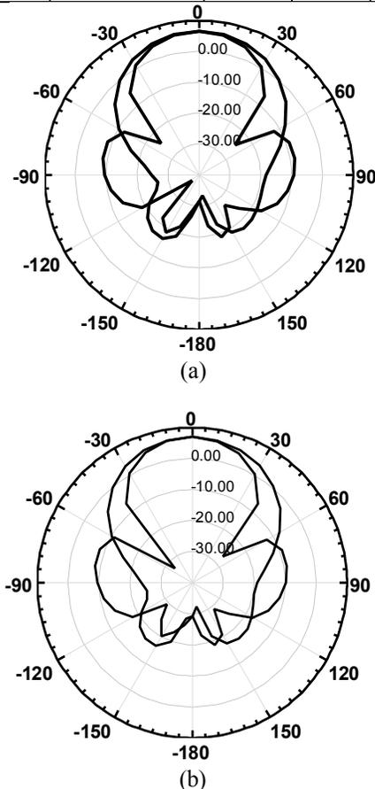
Figure 8. Radiation pattern of E plane (dash line) and H plane(solid line) for  $2 \times 2$  Circular polarized antenna with a ring of EBG a) near distance, b) far distance
