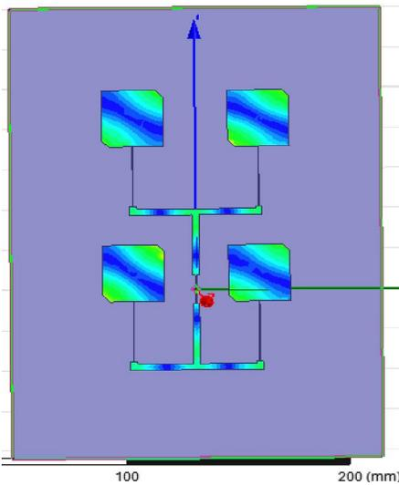
Figure 3. 2x2 Circular polarized antenna simulated using finite-element based HFSS to work at 2.48 GHz as shown in figure 3.
