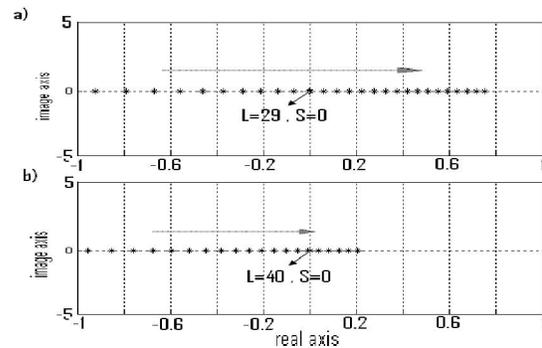
**Fig. 11.** The root locus of the dominant poles of the system in the stability margin during length increases and voltage ranges. a) 0.02 pu b) 0.05 pu.
