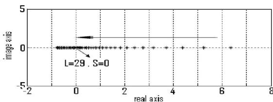
**Fig. 10.** The root locus of the dominant poles of the system for  $L=45$  and with a positive slope of active power-frequency droop characteristic.
