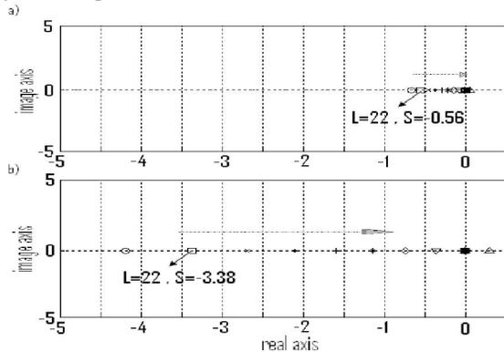
**Fig. 8.** root locus of the dominant poles of the system in the stability margin during length increases for allowed frequency ranges of. a) 0.2% and b) 1%
