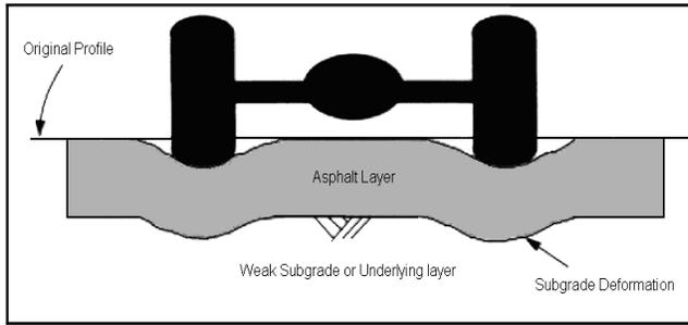
Fig 1. Rutting due to underneath layer deformation
