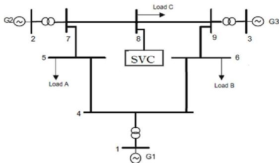
Figure 1. Multi-machine electric power system installed with SVC
