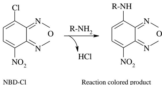
**Figure (2): The proposed reaction mechanism between NBD-Cl and primary amines**
