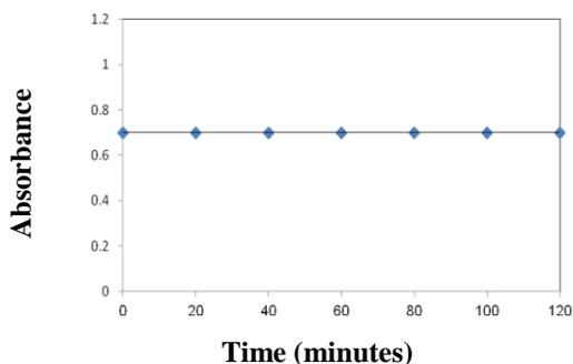
Figure (7): Effect of time on the stability of color of D-ZAF- NBD-Cl complex ( $2 \mu\text{g mL}^{-1}$ )
