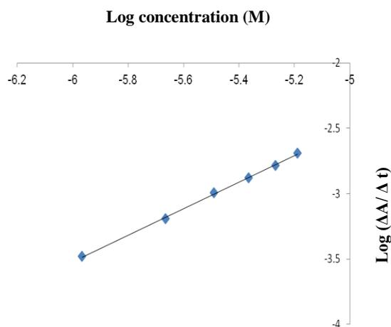
Figure (10): Calibration plot of logarithm rate of the reaction versus molar concentrations of hydrolyzed ZAF
