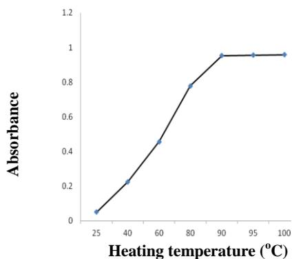
Figure (5): Effect of heating temperature on the reaction of degraded zafirlukast ( $2 \mu\text{g mL}^{-1}$ ) with NBD-Cl
