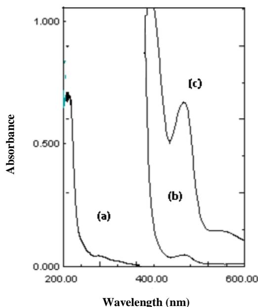
**Figure (3): Absorption spectra of (a) zafirlukast hydrolysate ( $2 \mu\text{g mL}^{-1}$ ), (b) reagent blank and (c) the reaction colored product.**
