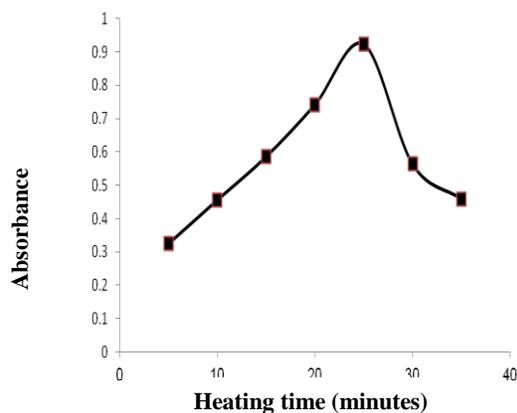
Figure (6): Effect of heating time at  $90^{\circ}\text{C}$  on the reaction of degraded ZAF ( $2 \mu\text{g mL}^{-1}$ ) with NBD-Cl
