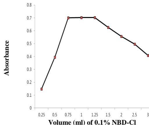
**Figure (4): Effect of volume of 0.1 % NBD-Cl on the reaction of zafirlukast ( $2 \mu\text{g mL}^{-1}$ ) after alkaline hydrolysis**
