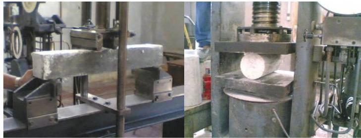
**Fig. 6: Plain Concrete Beam and Concrete Cylinders under Test****Testing equipment and loading arrangement**
