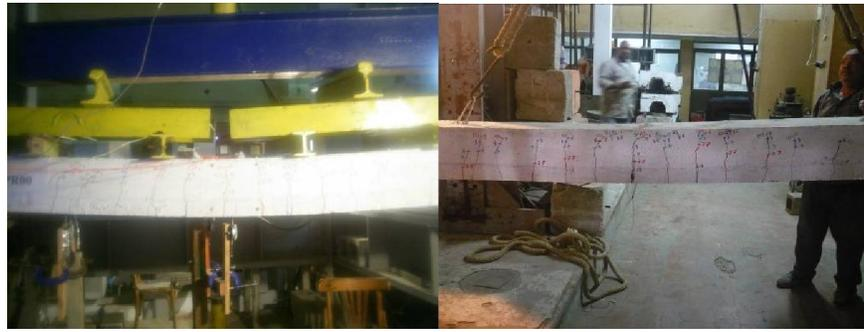
**Fig.9: Flexural Behavior of Specimen**
