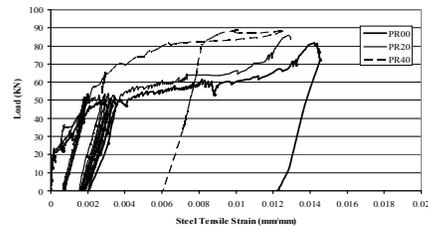
**Fig.14: Load Steel Tensile Strain Relationship for Slabs with Prestressed Concrete Precast Pane**
