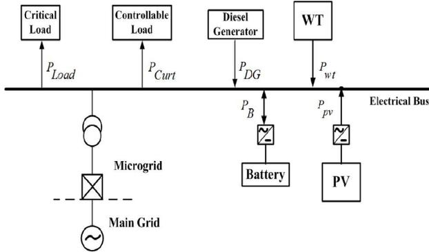
Fig. 1. Structure and direction of energy current
