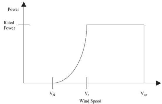
Fig. 2. Curvy of power-velocity of wind turbine
