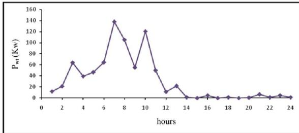
Fig. 7. Wind turbine output power in 24 hours
