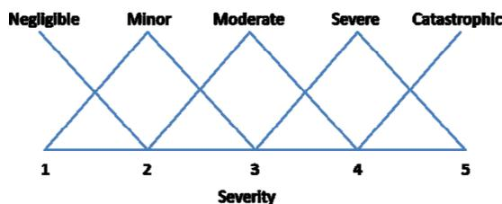
Figure 3. Fuzzy set for the definition of Severity
