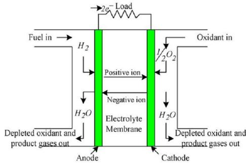
Figure 2)The overall schematic of fuel cell reaction
