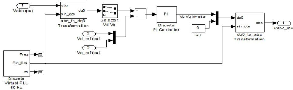
Figure 8) Voltage regulator diagram in simulink
