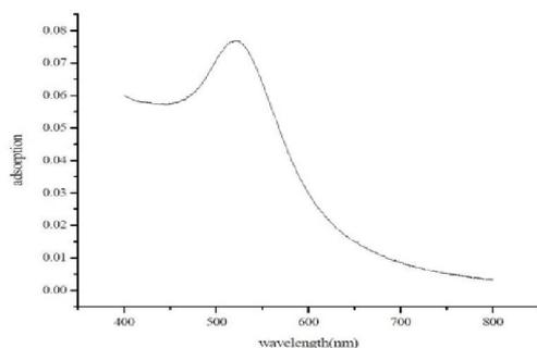
Figure (1) UV-vis spectroscopy of colloids gold nanoparticles
