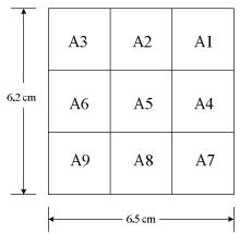
**Figure 2.** The sampling positions of the exposure area applied in the experiments. The diameter is about  $62 \times 65$  mm in the wedge bottom. The sampling positions of ultrasonic diathermy system is the same as this figure, only the exposure area of ultrasonic diathermy system is about  $30 \times 30$  mm.
