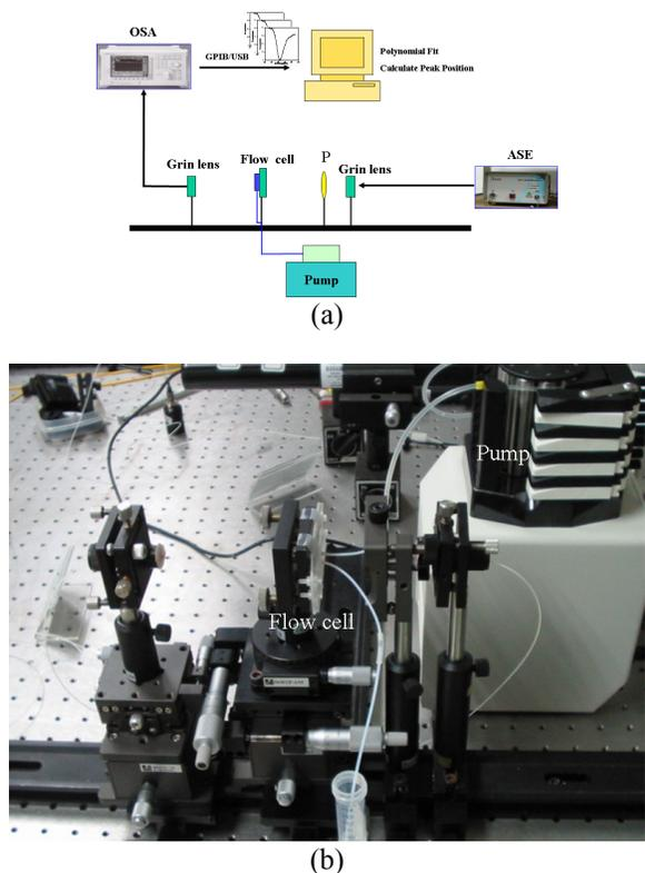
Figure 4. The experiment setup of DNA hybridization.
