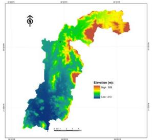
Fig 4: The SRTM DEM for Wadi Ibrahim catchment, location of The Holy Mosque is indicated by the black square.
