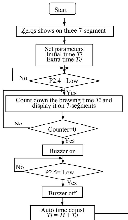
Figure 2. Flow chart of the software control codes.
