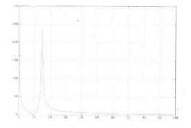
Figure 5.ELF signal at 15  $\rm H_z$  is identified by QT when 0.0001  $\leq$  S/N < 0. 3
