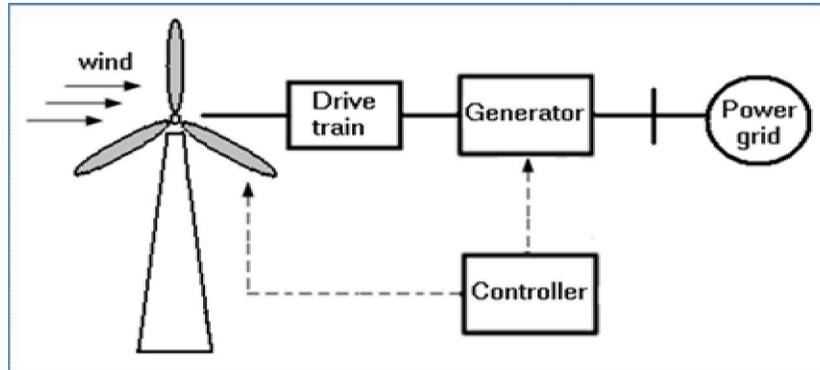
Fig. 6. Block Diagram of (DFIM) Wind Turbine
