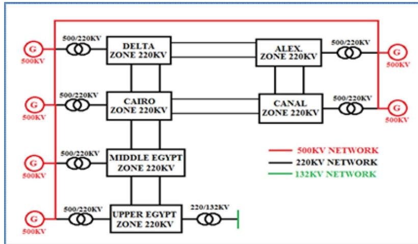
Fig. 1. Egypt Network (500kv, 220kv and 132kv)
