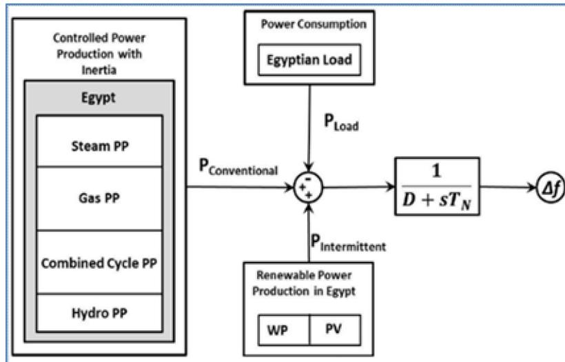
Fig. 5. Block Diagram of Power Balance for Egyptian Network
