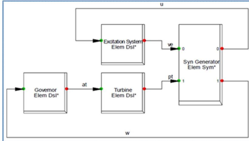
Fig. 4. Block Diagram of Composite Model
