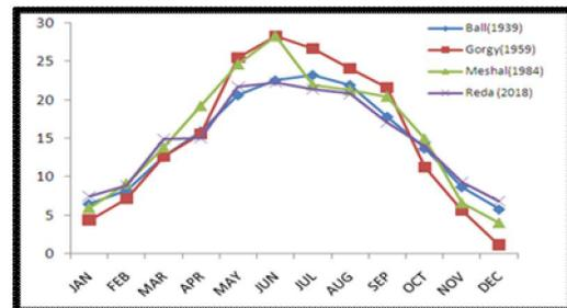
**Figure (2)** comparison between different methods for annual evaporation of Lake Qarun
