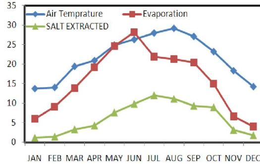
Figure (6) shows the effect of temperature and evaporation rate on extracted salts of Lake
