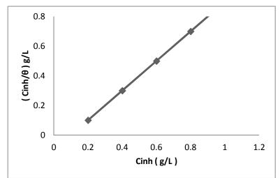
Fig. 2. Curve Fitting of weight loss data for aluminum electrode in HCl containing parsley extract to langmuri adsorption isotherm at 298 K.
