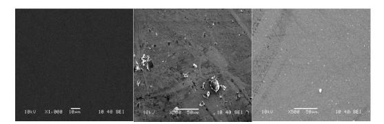
Fig.3. SEM image of aluminum electrode (a) polished, (b) immersed in 1M HCl and (c) immersed in 1M HCl containing 0.3 M Inhibitor.
