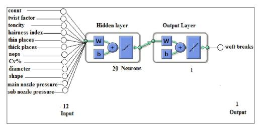
Fig. 1. First artificial neural network model (I).
