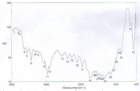
Figure 4: FTIR Spectrum of Plasma Oxygen treated Warp PET
