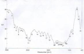
Figure 3: FTIR Spectrum of Untreated Warp PET
