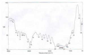
Figure 5: FTIR Spectrum of Plasma Air treated Warp PET
