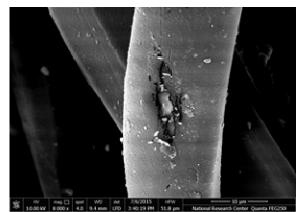
Figure 8: SEM of Plasma Air treated (8mA for 5min) F1
