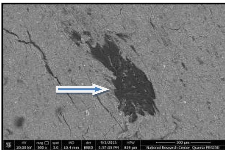
Fig. (6) The scanning electron microscopy of ungrafting paper written with erasable inks
