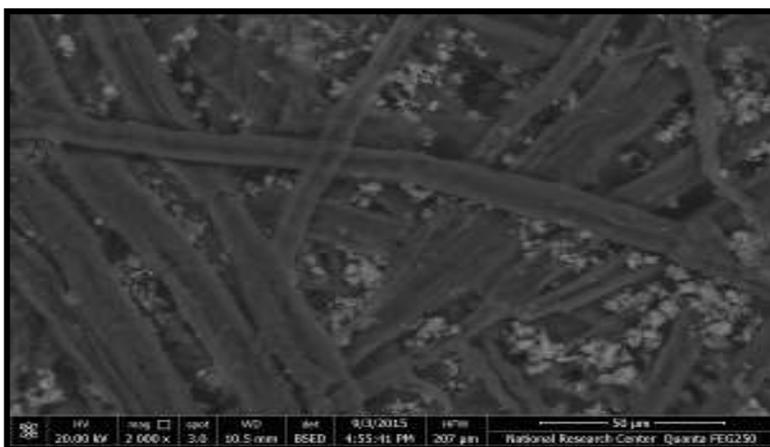
Fig. (7) The scanning electron microscopy of grafting paper only
