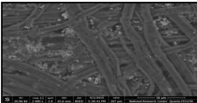
Fig. (8) The scanning electron microscopy of grafting paper written erasable inks then erased
