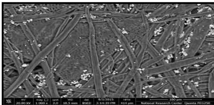
**Fig. (4) The scanning electron microscopy of blank paper**
