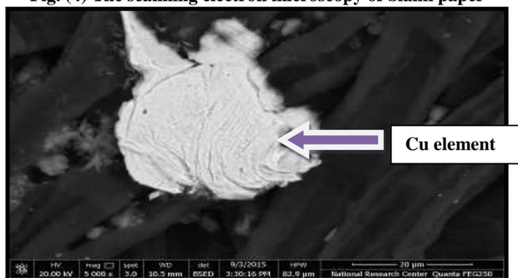
**Fig. (5) The scanning electron microscopy of blue ballpoint on paper**
