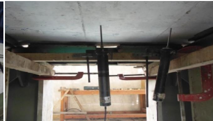
Fig (6): Locations of vertical LVDT'S
