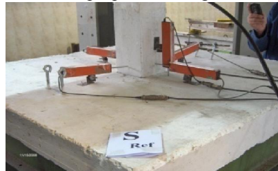
Fig (5): Locations of vertical LVDT'S
