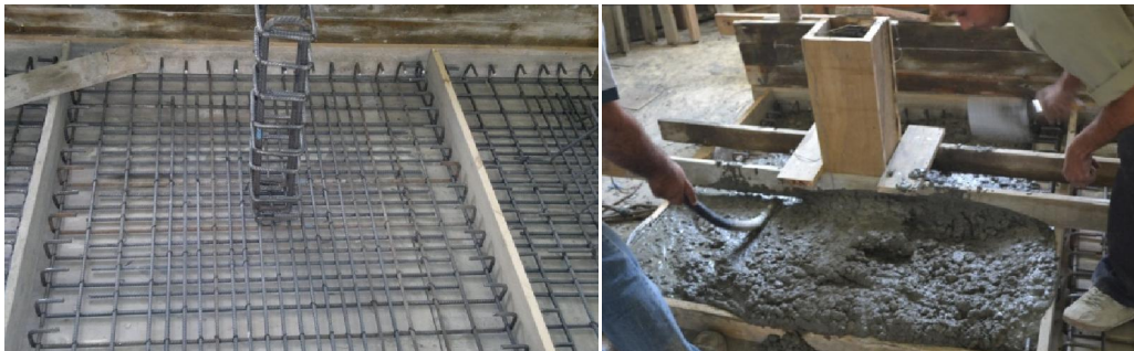
Figure (3): Details of Specimens Casting Forms
