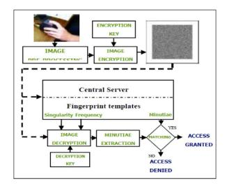
Fig.2. Schematic of embedded crypto biometric authentication system
