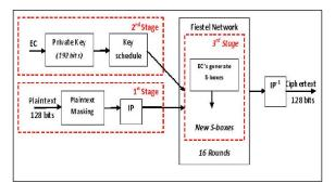
Fig.1. DES-EC Encryption Stages.
