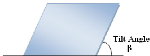
Figure.1 Tilt Angle of Photovoltaic Module
