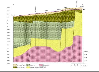
Figure 2. Aquifer configuration of Wadi Qena
