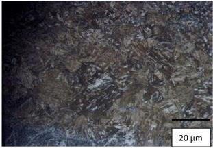
Fig. 8 microstructure at the heat affected zone (HAZ)
