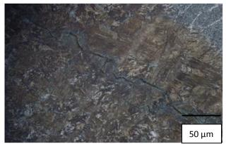
Fig. 9 Microstructure at the cracked HAZ
