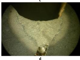
Fig. 4 Macrostructures of the cross sections of cold cracking test using a) Welding without drying, b) Welding with drying at 300  $^{0}$ C for 2 hours, c) Welding without drying and preheating at 150  $^{0}$ C and d) Welding with drying at 300  $^{0}$ C for 2 hours and preheating at 150  $^{0}$ C
