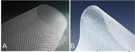
Fig. 1 A. Lightweight (40 gm/m<sup>2</sup>) and B. heavyweight (84-100 gm/m<sup>2</sup>) polypropylene mesh <sup>10</sup>.
