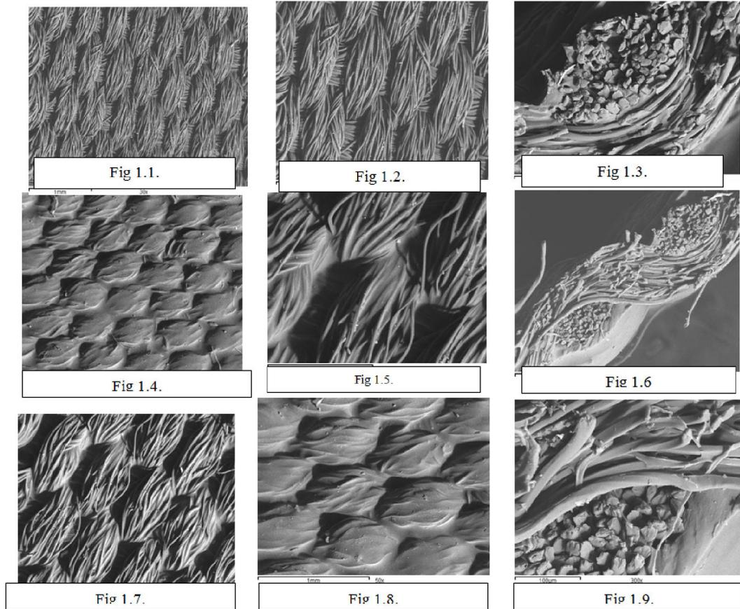
**Fig. (1)** Scanning electron micrograph (SEM) of plain weave sample before and after treatment
