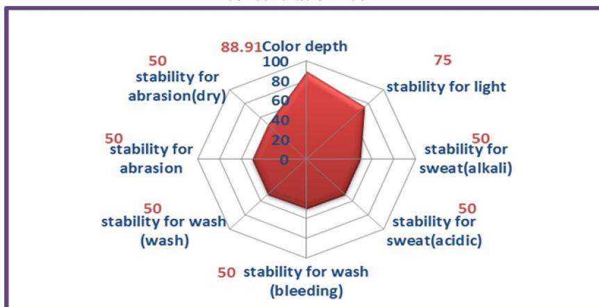
Figure (7) The best samples(sample no. 57) ring end spinning, time (1 minute), microwave energy 510, and dye concentration 2% R+
