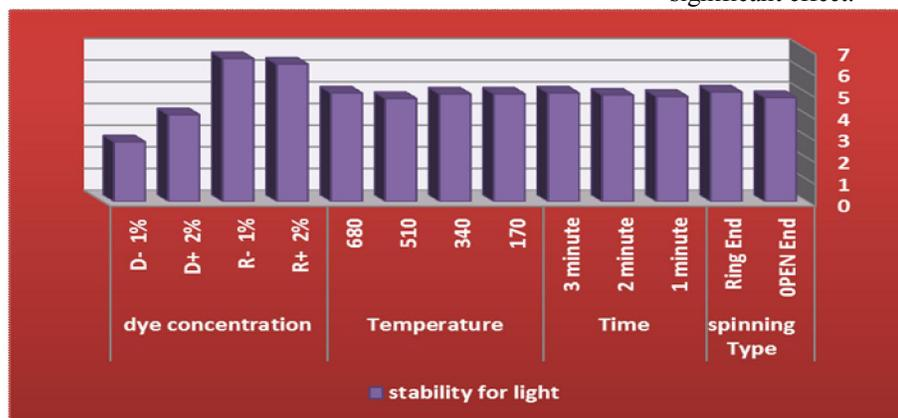
**Figure (5) Effect of Spinning type, time, microwave energy and concentration of dye on fastness against light**
