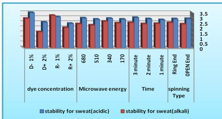
Figure 4. Effect of Spinning type, time, microwave energy and concentration of dye on fastness against sweat (acidic- alkali)
