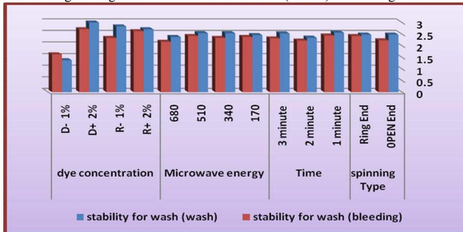
Figure 3 Effect of Spinning type, time, microwave energy and concentration of dye on fastness against washing (wash-bleeding)
