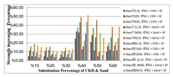
Fig (7) Percentage of Increasing Strength for substitution CKD, Sand and Silica Fume
