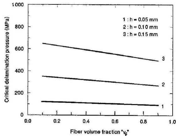
Figure (4) Critical delamination pressure versus fiber volume fraction at different values of uncut thickness.
