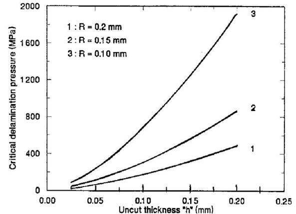
Figure (2): Critical delamination pressure versus uncut thickness at different values of water jet radii.
