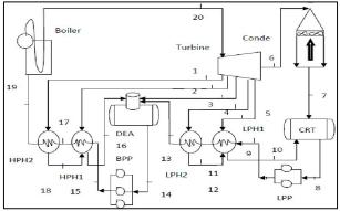
Figure 1 schematic flow diagram the steam power plant
