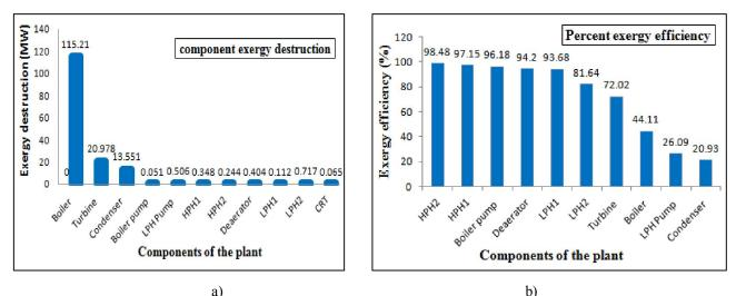
**Figure 2: (a)**Exergy destruction, (b) Exergy efficiency of every components of the plant
