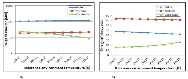
**Figure 3:** Effect of reference environment temperature on (a) the exergy destruction (b) the exergy efficiency of major plant components
