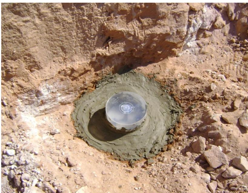
**Fig.2** Radon chamber set up in the field.
