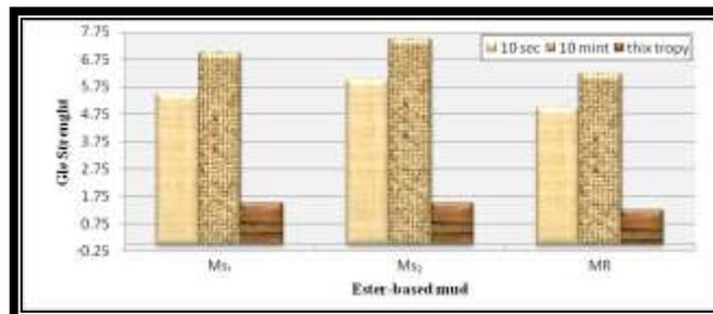
Fig.(7): Gel Strength of synthetic Esters-Based mud formulated with a new prepared esters ( $M_{S1}$ ,  $M_{S2}$ ), compared to refers sample ( $M_R$ )
