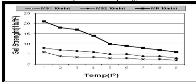
Fig.(12): G<sub>10</sub> min -Temperature relationship of synthetic Esters-Based mud formulated with a new prepared esters (M<sub>S1</sub>, M<sub>S2</sub>), compared to refers sample (M<sub>R</sub>)
