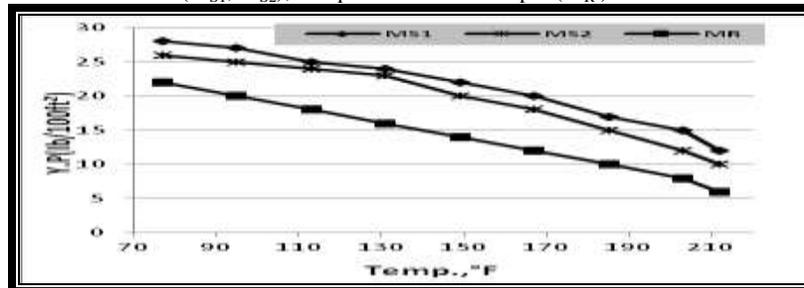
Fig.(10): Yield point (Y.P) -Temperature relationship of synthetic Esters-Based mud formulated with a new prepared esters ( $M_{S1}$ ,  $M_{S2}$ ), compared to refers sample ( $M_R$ )
