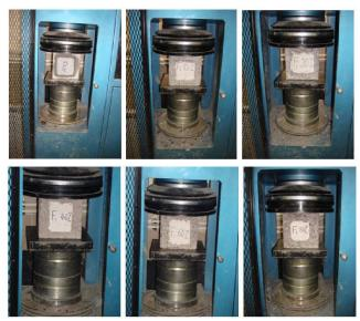
Fig. 5. Loading of cubic specimens with a percentage of 0, 10, 20, 40, 60 and 80, by total weight of the fine aggregate in concrete.
