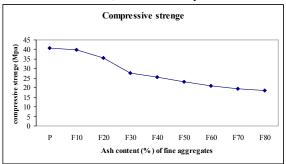
Fig.4.Compressive strength of concrete containing Ash particles.
