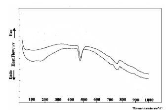
Figure 6: DTA thermgrams of E0 and E3 suspensions after 24hours
