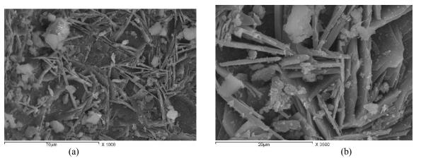
Figure (3) SEM micrographs of E0 suspensions 0a)- after 6 hours, (b)- after 24 hours.
