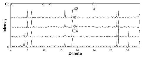
Figure (2): X-ray after 24 hours, g- gypsum, e- ettringite, C -CaO
