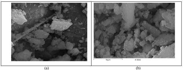
Figure (4): SEM micrographs of E4 suspensions (a)- after 6 hours,( b)- after 24 hours.
