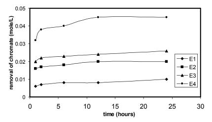
Figure (7): Removal of chromate ions of different mixes
