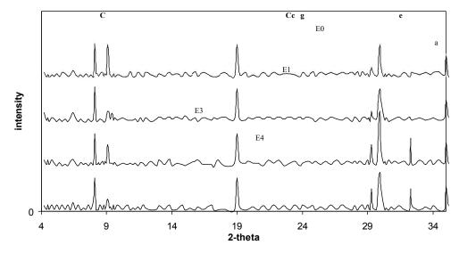
Figure (1): X-ray after 6 hours, g-gypsum, e- ettringite, C -Ca O , a- Al<sub>2</sub>(SO4)<sub>3</sub> Cc - CaCO<sub>3</sub>
