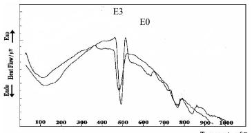
Figure 5: DTA thermgrams of E0 and E3 suspensions after 6 hours
