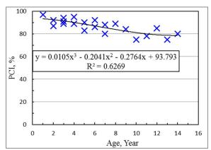
Figure 9: Family Curve for Concrete pavement
