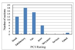
Figure 6: Number of Sections by PCI
