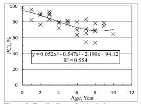
Figure 8: Family Curve for Asphalt pavement
