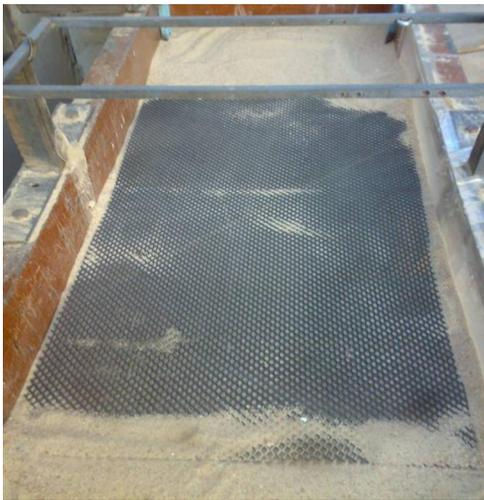
Fig. 3 Photographic view of Geogrid reinforcement.
