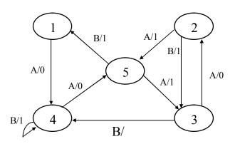
Figure 1: A Transition Diagram for a Machine M
