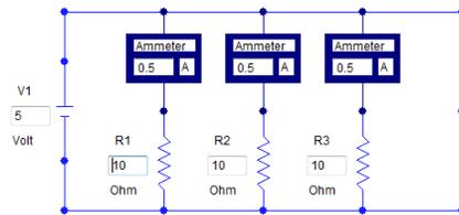
(e) Parallel connection of resistors.
